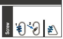
WARNING! If the lanyard is equipped with SCREW locking carabiners, please make sure that the gate is fully closed and tightened correctly, before using it! Note: SCREW locking carabiners shall NOT be used at workplaces where the user must connect/disconnect frequently! If the lanyard is equipped with AUTO-LOCK, TRI-
