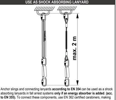
to EN 355). To connect these components, use EN 362 certified carabiners, making sure the length of the assembly does NOT exceed 2m! Before starting the work, make sure there is enough free space below the workplace! Read carefully the instructions of each component of your system!
